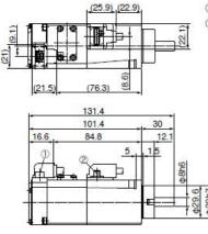
① Encoder connector 2 Motor/Brake connector
